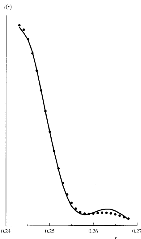
Fig. 10. Comparison of calculated and observed diffraction profiles. The solid line is a 110 reflection by polyethylene fibers, taken from Hall & Somashekar (1991). The dots represent the calculated diffraction using the size and the degree of disorder measured by the single-peak technique.
